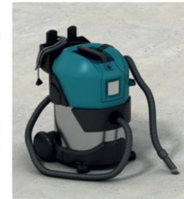
Vacuum debris and dust to ensure a clean surface.
